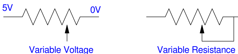
Two common configurations for potentiometers
