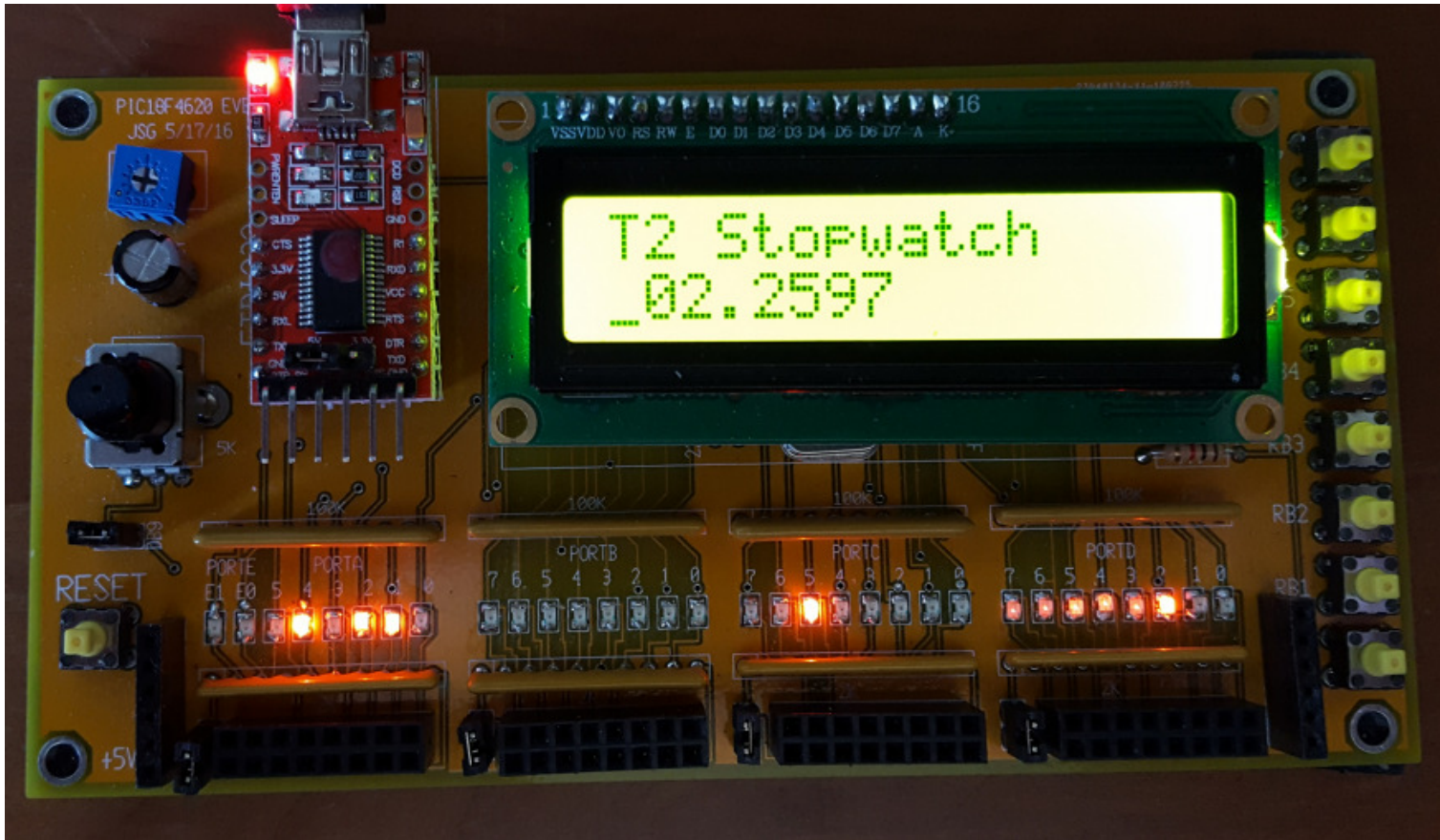
LCD Display of Time, Accurate to 0.0001s (one interrupt)
