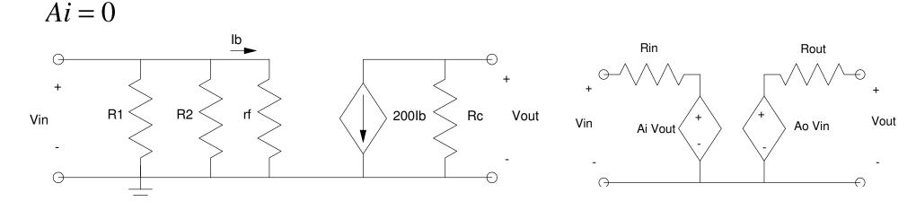
**Rout:** For the 2-port model, short Vi so that Vi=0 and  $A_oV_{in}=0$ . Measure the resistance at the output. Doing the same for the CE amplifier, this results in
