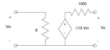
Note that the common-base amplifier has a low input impedance. It's used as the first stage in an amplifier where the sensor needs a low-impedance load, such as a phonograph (the current carries the signal.)
