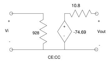
Common collector amplifiers are used as the last stage for an amplifier when you need to drive a low-impedance load, such as an 8-Ohm speaker.
