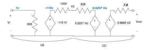
Solve for the voltage at V2. Using voltage nodes:
