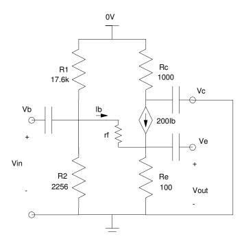
To find the 2-port parameters, redraw the circuit:
