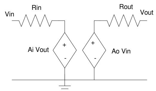
**7. 2-Port model (experimental):** Determine the 2-port parameters for an unknown circuit (shown in blue) given the following experimental data:
