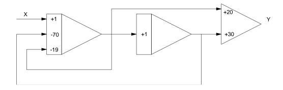
Adjusting the gains so they are all negative. Add an inverter when needed
