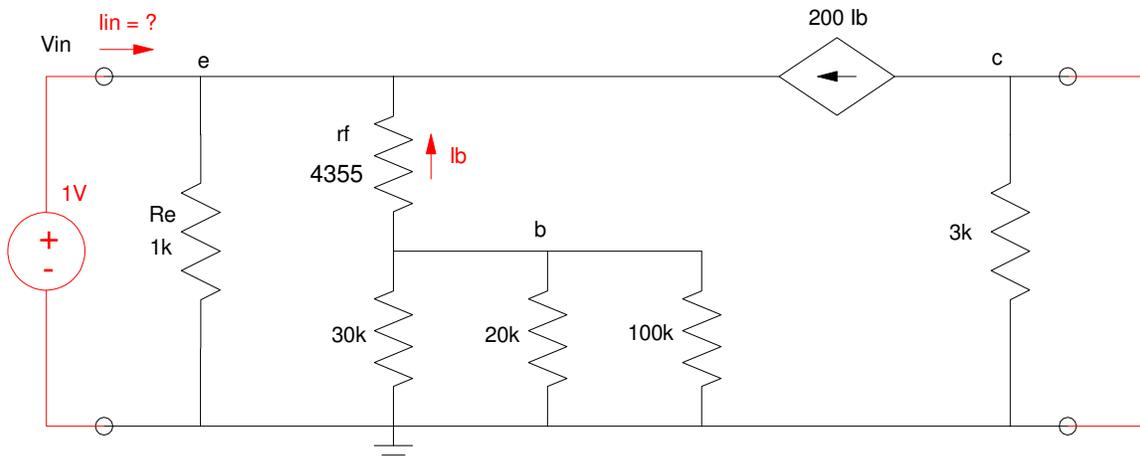
$$I_{in} = \frac{1V}{1k} + \frac{1V}{4355 + 30k \parallel 20k \parallel 100k} + 200 \left( \frac{1V}{4355 + 30k \parallel 20k \parallel 100k} \right)$$
