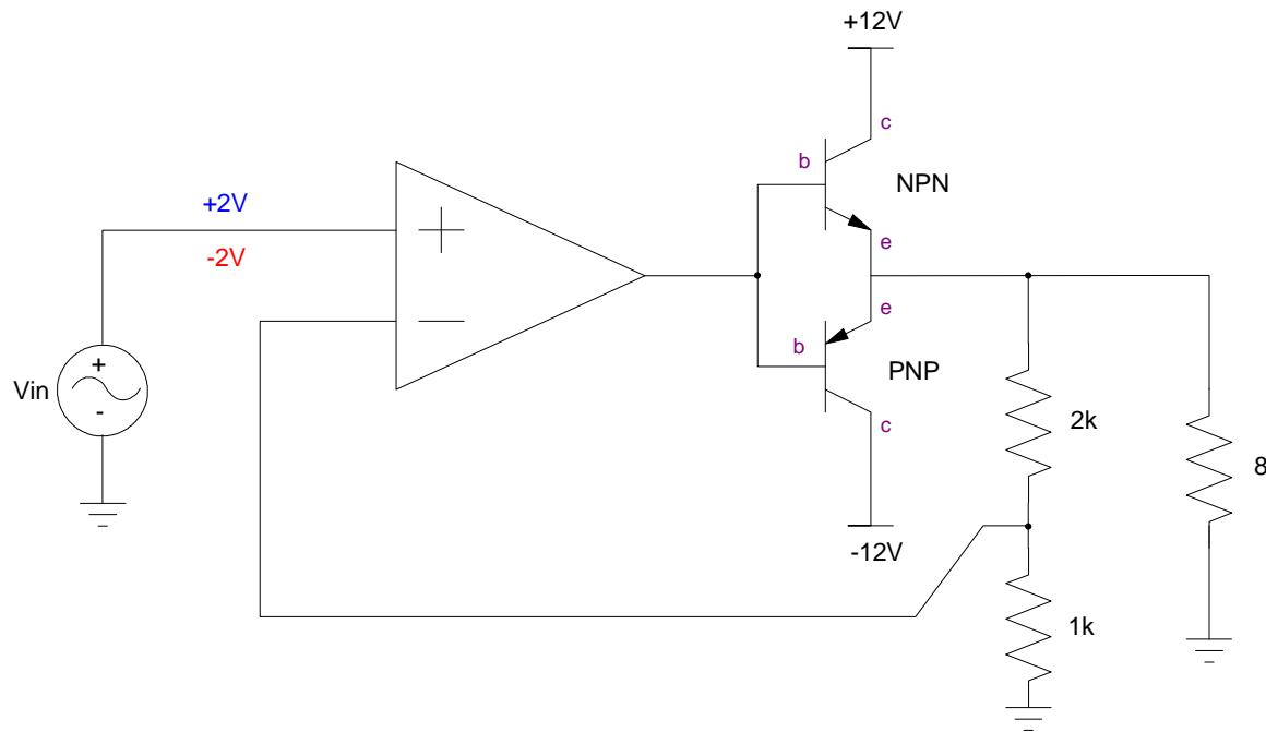
**Current Amplifier:** Find the voltages and currents for  $V_{in} = \{ +2V, -2V \}$
