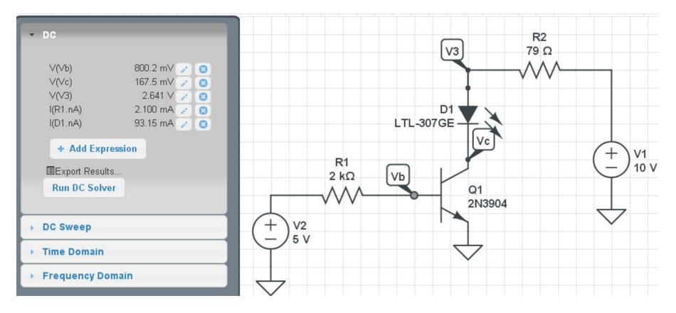
Note that Vce = 167mV tells you that the transistor is saturated:
