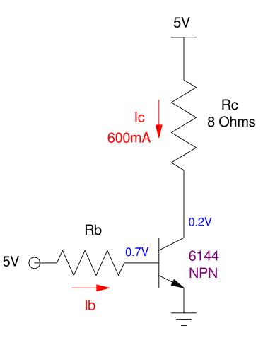
Step 3: Determine Ib ( assume Ib < 25mA )
