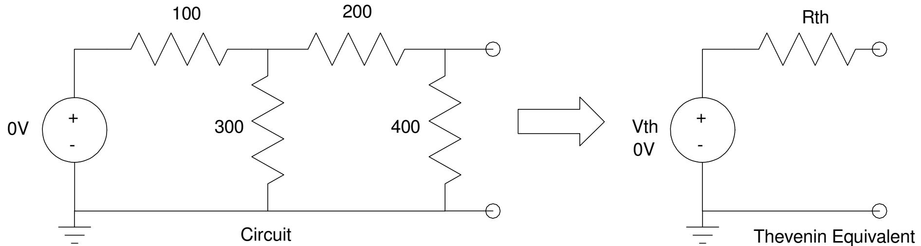
R<sub>th</sub> (take 2): Sometimes the resistance looking in isn't obvious. In that case, apply a 1V test voltage and compute the current. The Thevenin resistance is then
