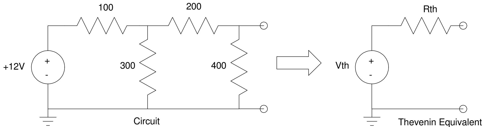
Since the two circuits are equivalent, whatever test you do on the circuit to the right to find  $V_{th}$  and  $R_{th}$ , do the same test to the original circuit.
