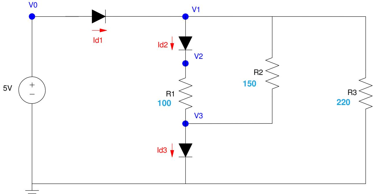
8) Write the voltage node equations assuming nonlinear diodes. Solve for {V1, V2, and V3} using Matlab.
