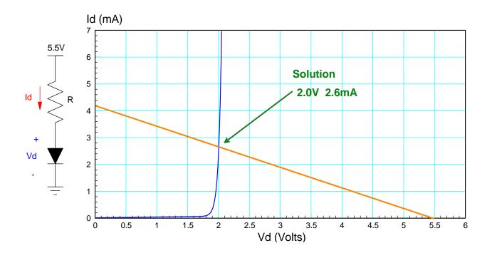
5) Diodes (nonlinear equations): Assume the VI characteristics of a diode are
