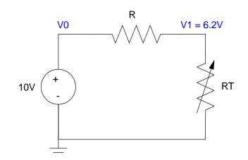
$$V_1 = \left(\frac{R_T}{R_T + 1314}\right) V_0$$
