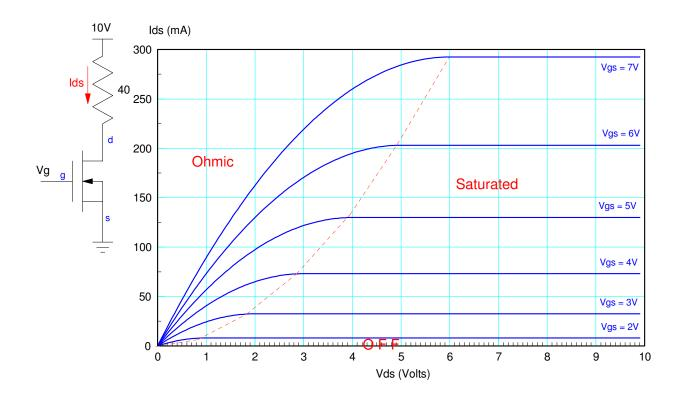
2) Draw the load-line for the circuit below. From the load line, determine the Q-point (Vds, Ids) when
