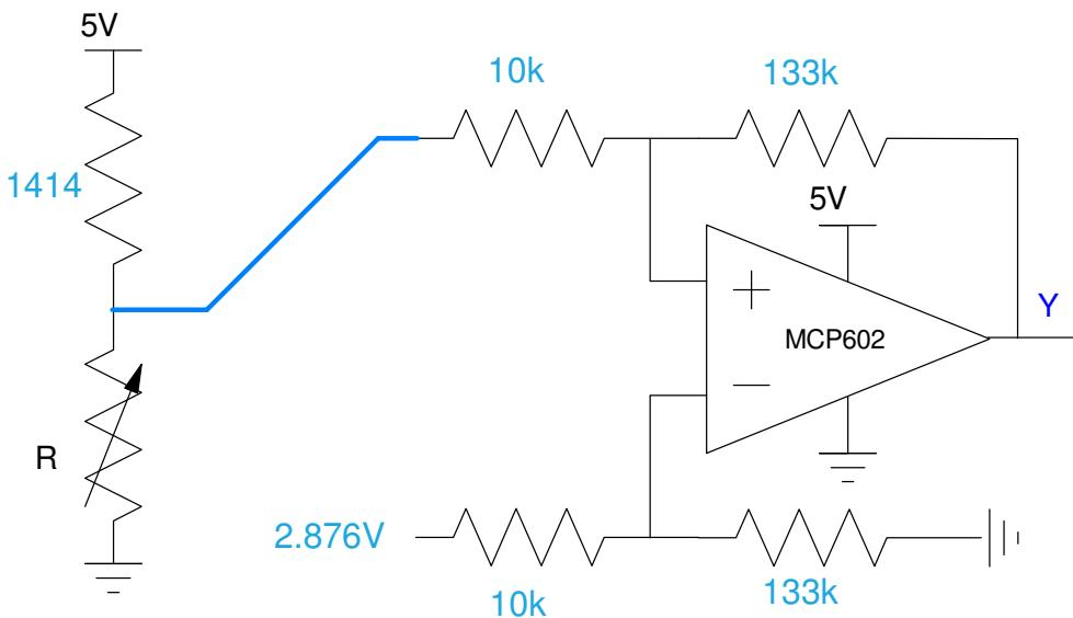
6) Schmitt Trigger: Analysis. Determine the voltages and resistance where the following Schmitt trigger turns on and off. Assume Rx is  $900 + 10^*(\text{Birth Month}) + (\text{Birth Day})$ .
