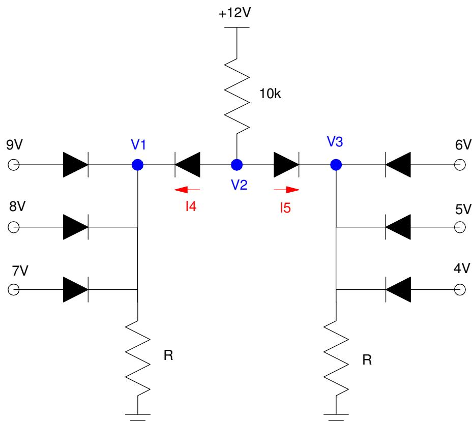
2) Max/Min: Determine the voltages and currents for the following min/max circuit.
