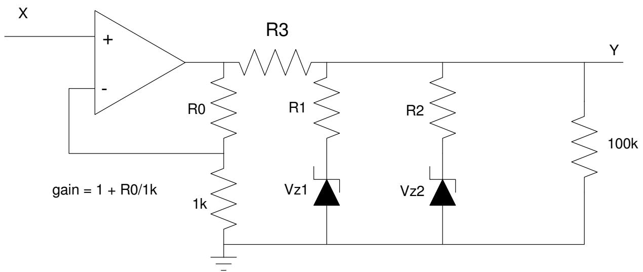
4) Clipper: Design a circuit to clip the voltage at +8V and -7V
