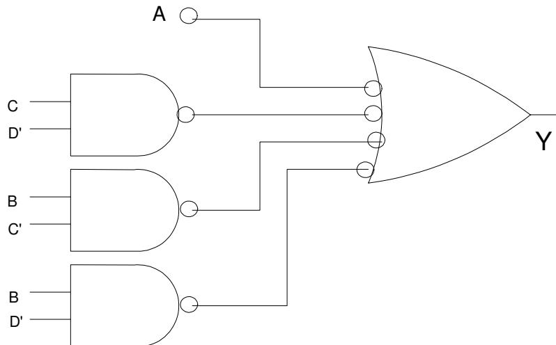
2) Implement the following function using NOR gates (i.e. circle the zeros)
