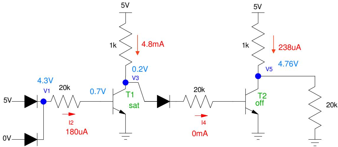
The 5V source turns on transistor T1 (saturated)
