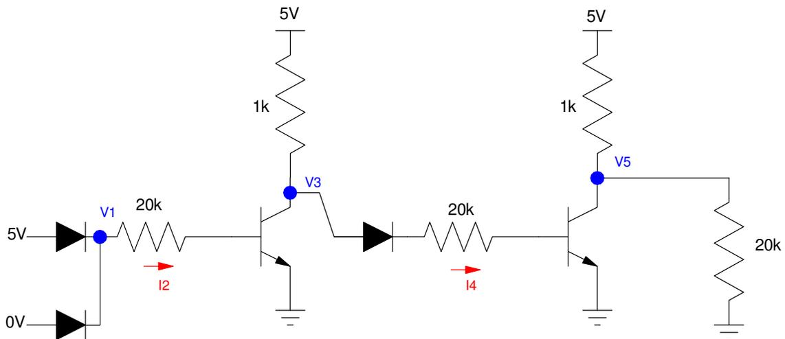
The circuit below uses a DTL NAND gate to drive the speaker when
