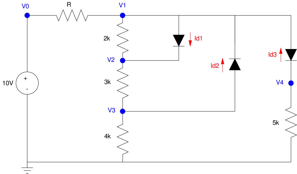
3) Ideal Silicon Diodes. Assume the diodes in this circuit are ideal silicon diodes:
