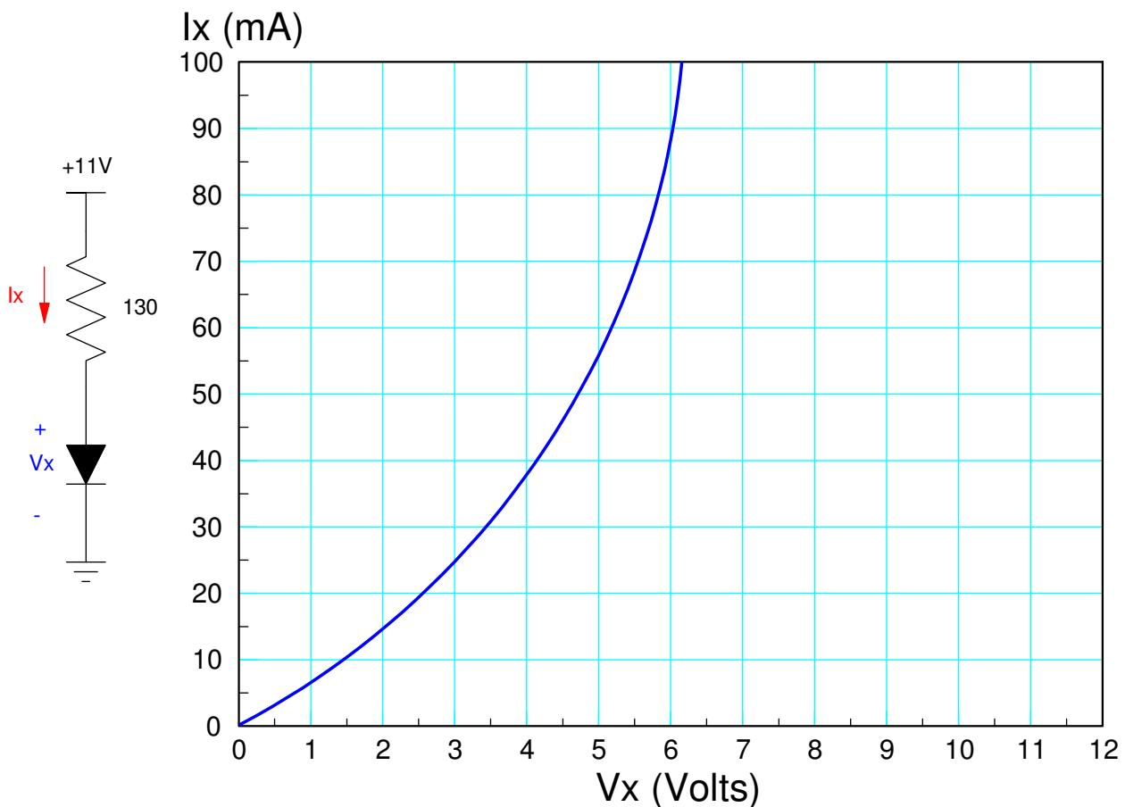
2) Nonlinear equations: Diode circuit
