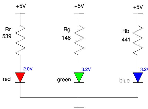
2) Design a circuit to drive these LEDs with a 5V source producing Cobalt Blue:
