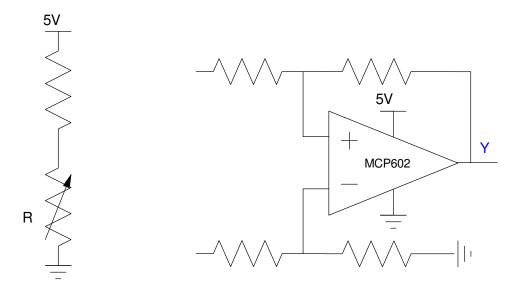
6) Schmitt Trigger: Analysis. Determine the voltages and resistance where the following Schmitt trigger turns on and off. Assume Rx is  $1000 + 10^{\circ}$ (Birth Month) + (Birth Day). May 14th gives Rx = 1514 Ohms.
