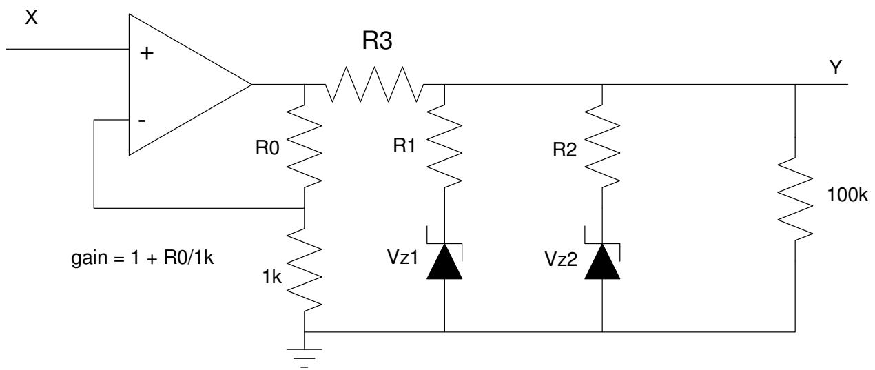
4) Clipper: Design a circuit to clip the voltage at +7V and -3V
