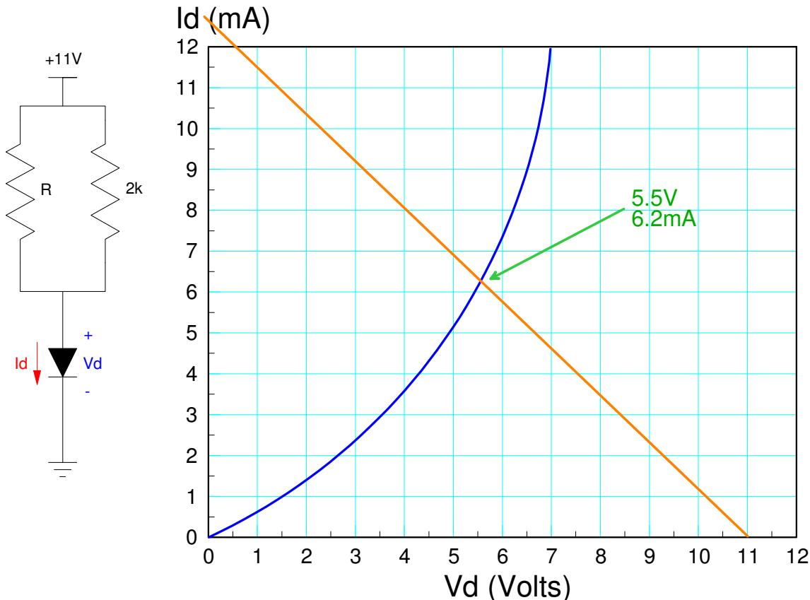
2) Nonlinear equations: Diode circuit
