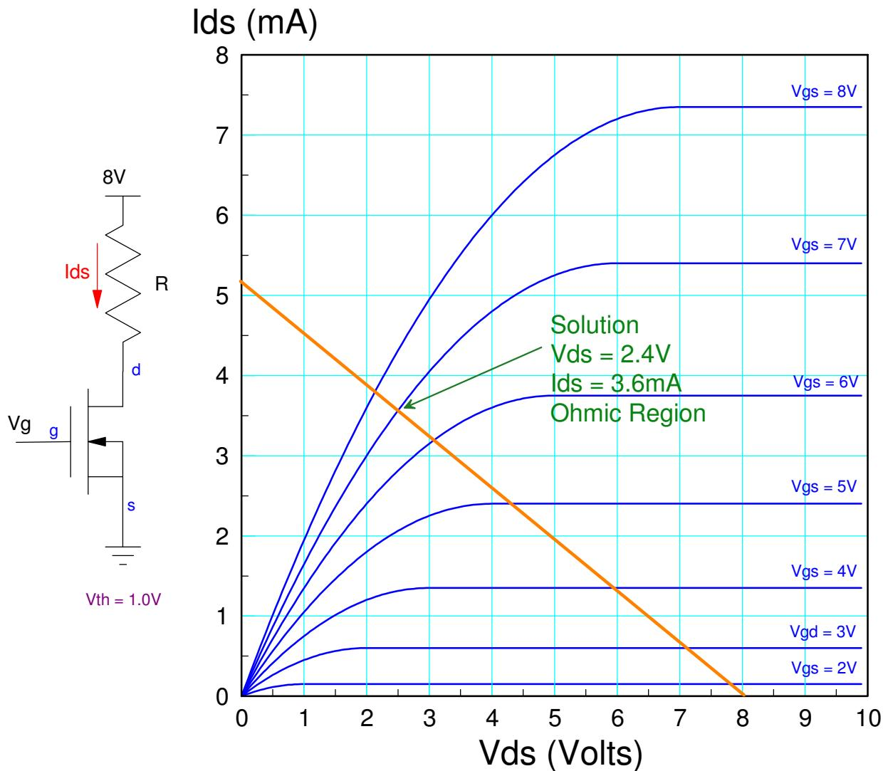
$k_n$  calculations: Pick a point ( $V_s = 10V$ ,  $V_{gs} = 8V$ ,  $I_{ds} = 7.3mA$ ) . Region = saturated
