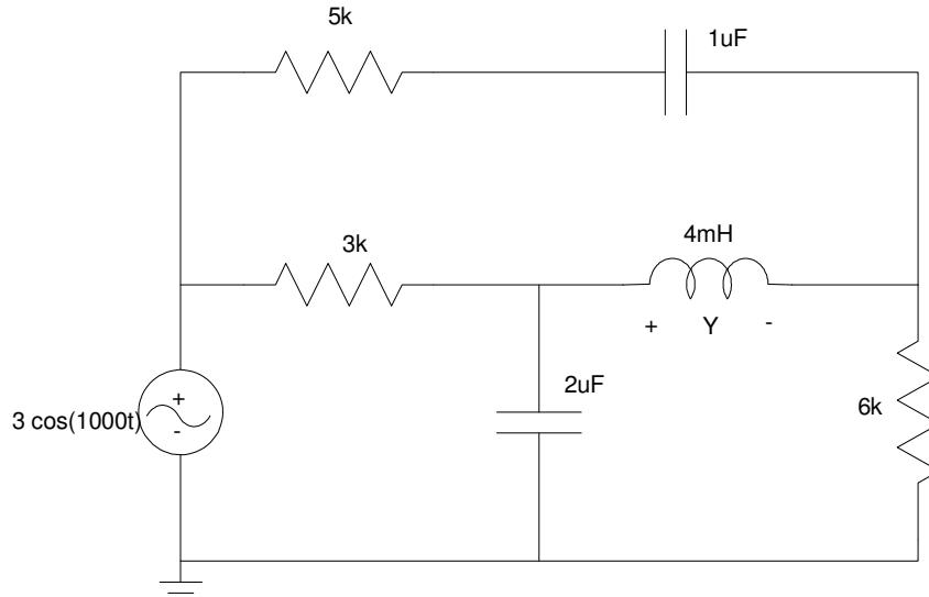
Example 1: Solve the following RLC circuits using current loops and voltage nodes.
