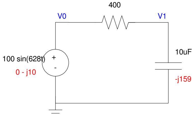
Step 1: Replace the voltage source and capacitor with their phasor value:
