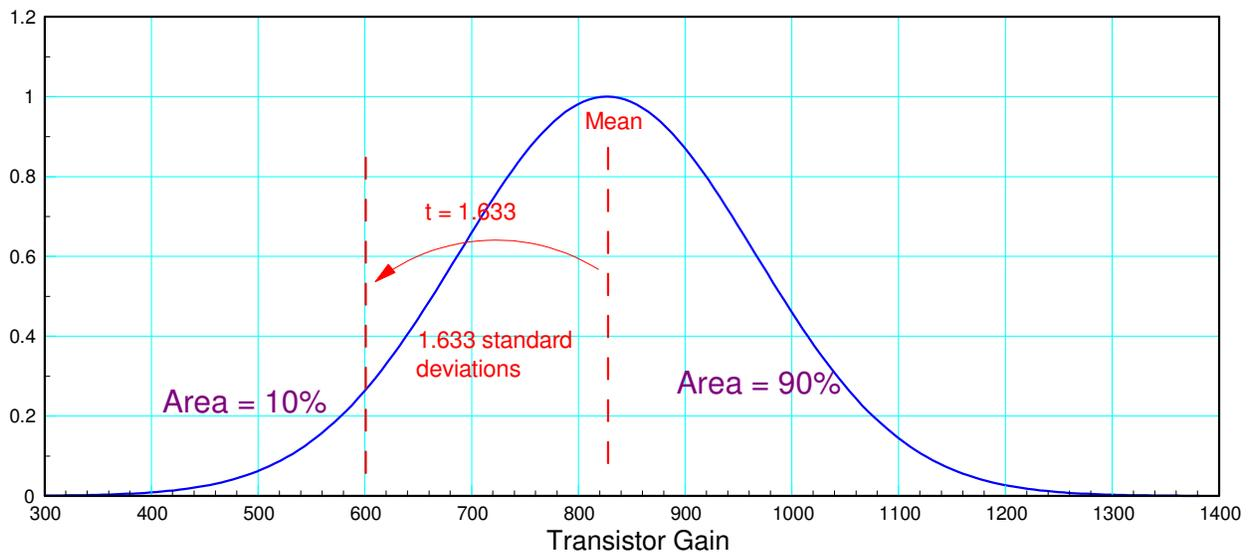
pdf of transistor gain. 90% of the area is to the right of 600
