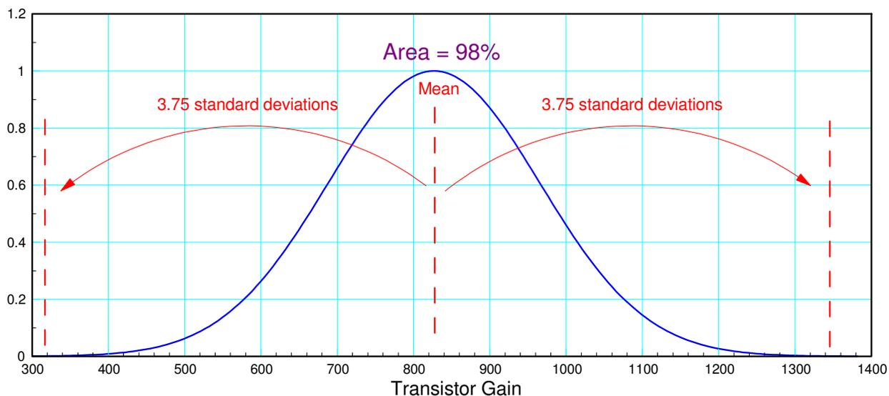
98% Confidence Interval: 98% of transistors should have a gain in the range of (305.9, 1348)
